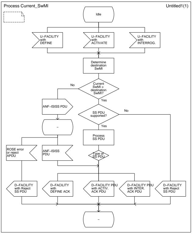
NOTE: Every ANF-ISISS PDU or ROSE APDU is conveyed by a PSS1 FACILITY message. The latter has not been shown in the corresponding signal symbols.
